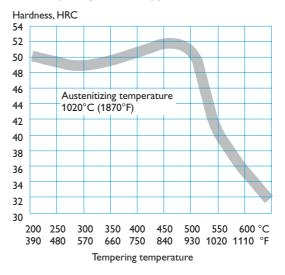
Above tempering curves are obtained after heat treatment of samples with a size of  $15 \times 15 \times 40$  mm, cooling in forced air. Lower hardness can be expected after heat treatment of tools and dies due to factors like actual tool size and heat treatment parameters.
