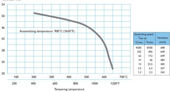
The curve represents a quenching speed of 60°/min. (140°F/min.) Tempering 2+2h.
