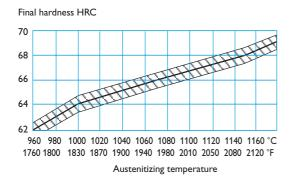
Hardness for different austenitizing temperatures after tempering 3 times for 1 hour at  $560^{\circ}$ C ( $1040^{\circ}$ F)  $\pm 1$  HRC.
